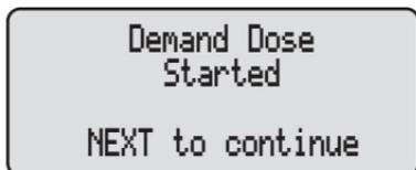
The pump will begin delivering the dose. When the Main Screen is displayed, **DOSING** will appear.
