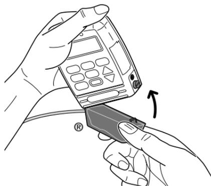
4. Insert the side of the key or a coin into the latching button, push in, and turn counterclockwise until the mark on the latch lines up with the solid dot.
